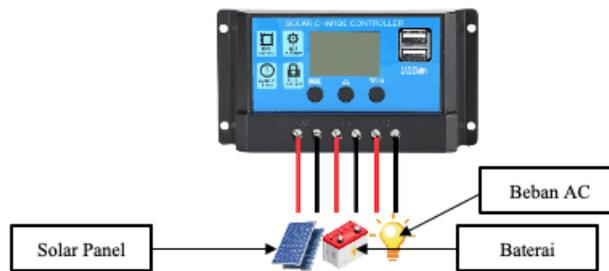
Gambar 28. Desain solar charge control
