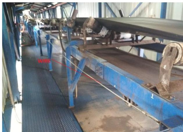
Gambar 8. *Wire pull cord switch*
