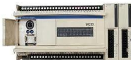
Gambar 2. PLC schneider twido [5]
